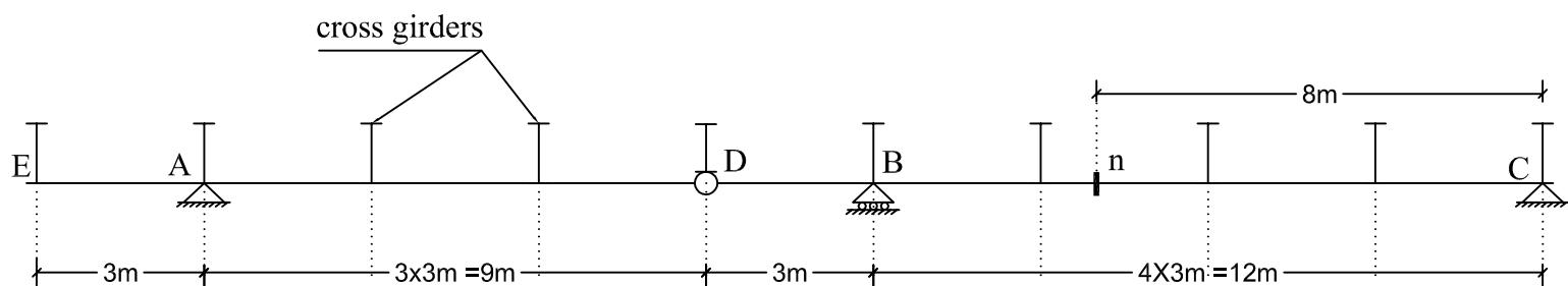
(3) I.L  $Y_A, Y_B, Y_C, Y_D, M_B, Q_n, M_n, Q_B$  left, and calculate  $M_{n \max}, M_{n \min}, Q_{n \max}, Q_{n \min}$ .
