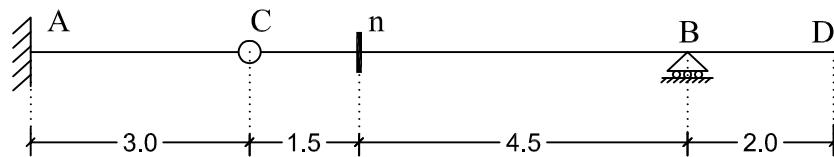
(1) I.L  $Y_A, Y_B, Y_C, M_A, Q_n, M_n, Q_B$  left, and calculate  $M_{n \max}, M_{n \min}$ .
