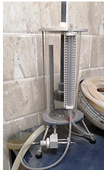
Jet Trajectory and Flow through Submerged Vertical Orifice Nozzle
